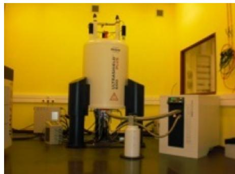
**Bruker Avance II+ 600 equipped with a TCI cryoprobe**
