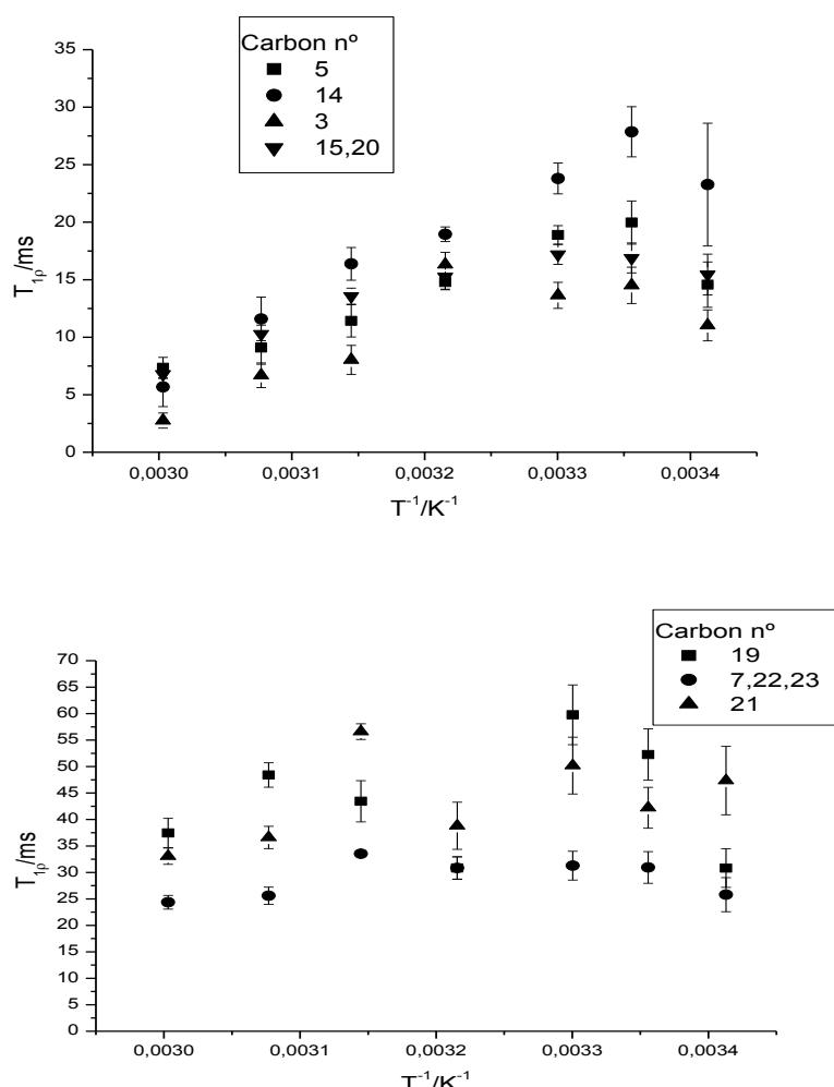
**Figure 2.** Spin-lattice relaxation time in the rotating frame of the indicated carbon atoms measured from 293 till 333 K.
