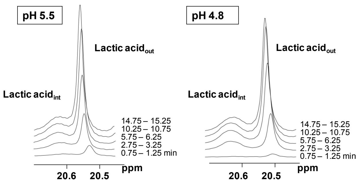
**Fig. 1.** Sequences of <sup>13</sup>C-NMR spectra obtained during glucose metabolism at external pH values of 5.5, and 4.8, showing two resonances, assigned as intracellular and extracellular lactic acid.
