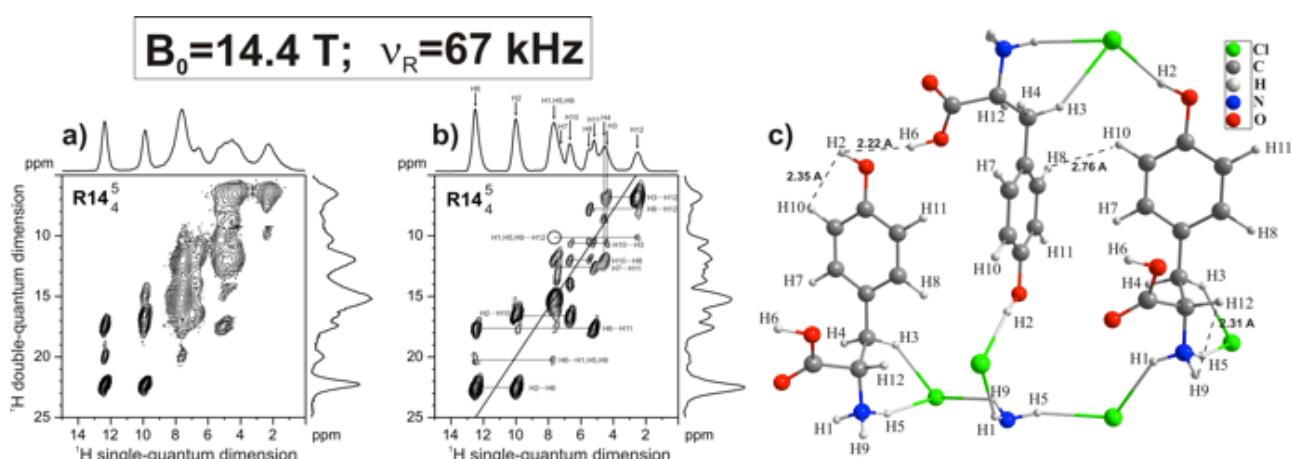
**Figure 3** – 2D  $^1\text{H}$ - $^1\text{H}$  DQ-SQ spectra of Tyr.HCl, recorded at MAS 67 kHz using  $v_1=117$  kHz and Larmor frequency of 600 MHz ( $B_0=14.1$  T, Bruker wide-bore NMR spectrometer), using the symmetry ??? for  $^1\text{H}$ - $^1\text{H}$  recoupling. a) No CRAMPS used, b) DUMBO decoupling in both dimensions (DUMBO shape pulse length = 15  $\mu\text{s}$ ; Decoupling power=198 kHz), c) Schematic representation of the solid-state structure of Tyr.HCl.
